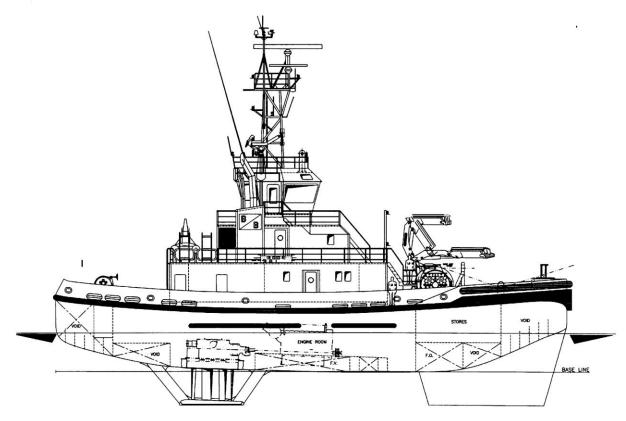
Fin First Voith Tractor Type: **Built:** 1999 Call sign: LJXK IMO no.: 9191905 Port of registration: Brevik DNV +1A1- E0 - Ice 1C - Tug Class: Escort (87,10;76,8) **Tonnage:** 436 GRT Speed: 14,2 knots **Bollard pull at MCR:** 48 tonnes Steering pull at 10 knots, in compliance with DNV class notation: 87 tonnes Main dimensions: 32.40 m Loa Bmld 11.40 m Dmld 4.80 m Normal op. draft 4.60 m
