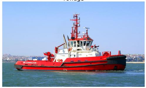
**Azimuth Stern Drive** Main engines: 2 x ABC 8DZC Type: **Built:** 2008 5.100 bhp in total Call sign: **LCBF Propulsion:** Azimuth CPP **Bow thruster:** IMO no.: 9451549 215 hp **Auxiliaries:** Port of registration: 350 kW Oslo Class: BV I+Hull+Mach Tug; FiFi I Fire fighting: 1 x water / foam monitor Unrestricted Navigation AUT UMS; 1 x water monitor SYS NEQ1 Escort (70, 10) 2.400 m<sup>3</sup>/hr water
