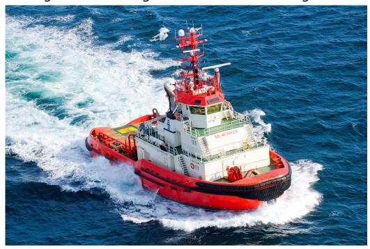
AHT / Azimuth Stern Drive Main engines: 2 x 2250 kW (Wärtsilä) Type: **Built:** 2007 **Propulsion:** Azimuth x 2 (Wärtsilä Lips) Call sign: **LNSA** Bow thruster: 1 x Pumpjet 350 kW **Auxiliaries:** 2 x 290 kW IMO no.: 9360051 Port of reg.: Stavanger
