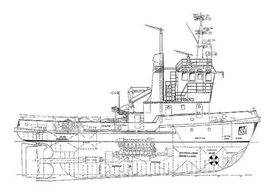
Type: Conventional **Built:** 1975 Call sign: **JXFF** 7406930 IMO no.: Bergen Port of registration: DNV +1A1 - R280 - E0 - Ice C - Tug Class: 181 GRT Tonnage: Speed: 12 knots **Bollard pull at MCR: 35 TBP** Main dimensions: Loa 26.68 m Bmld 8.23 m Dmld 4.20 m
