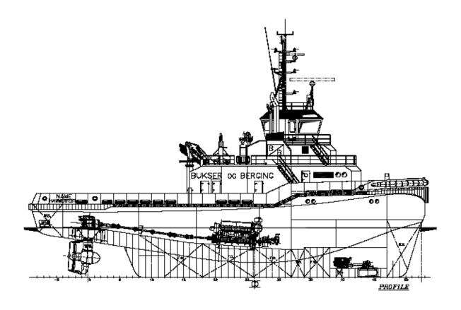
Type: Azimuth Stern Drive **Built:** 2006 Call sign: **LNND** IMO no.: 9334777 Port of registration: Hammerfest Class: DNV +1A1 - E0 - Ice C -Tug - SF - FiFi I - Oil rec 731 GRT Tonnage: Speed: 15 knots **Bollard pull at MCR:**
