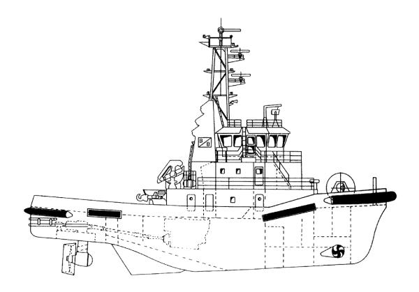
Type: Azimuth Stern Drive **Built:** 1991 Call sign: LJUO IMO no.: 9008641 Port of registration: Tønsberg Class: LR +100A1 - Tug - Ice 1C Tonnage: 344 GRT Speed: 14 knots **Bollard pull at MCR: 53 TBP** Main dimensions:
