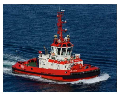
Type: Azimuth Stern Drive Main engines: 2 x CAT 3512C 4.080 bhp in total
